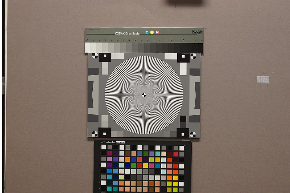
Figure 2. Typical image of Siemens star, framed so the maximum frequency is slightly above f_{Nyq} .
